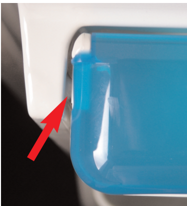
Gap between shelf and inner door.
