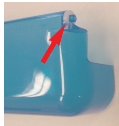
Put as many washers as you need on the hinge pin of the cover.
