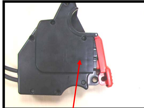
Old Level switch box.
